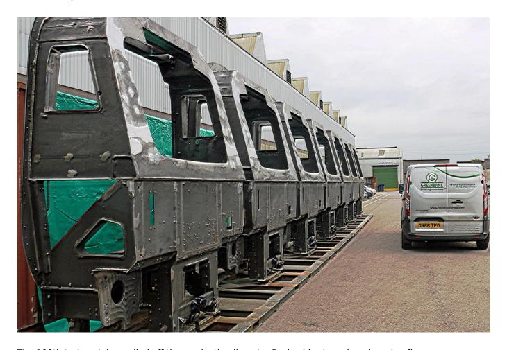
The 100th train cab has rolled off the production line at a Derbyshire-based engineering firm.
