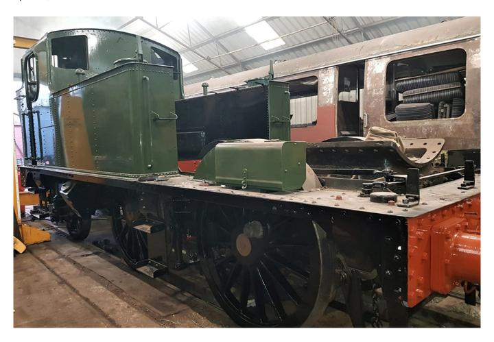
Work on the Great Western Society's first locomotive, No 1466, is continuing at Western Steam Engineering with the iconic GWR 0-4-2T on track to return to steam at Didcot Railway Centre later this year following the most extensive overhaul she has received since 1961.
