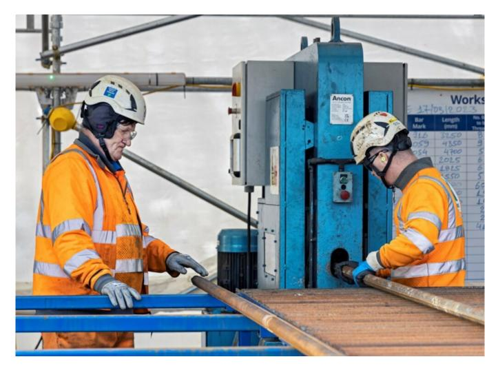
HS2 has set up a rebar threading facility to address materials shortages at its Copthall tunnel construction site in Hillingdon – creating jobs, cutting waste and reducing lorry movements. The new facility will make 92,000 rebar couplers, needed to construct the Copthall tunnel.
