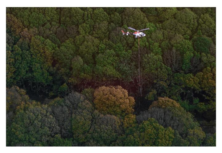
In partnership with Tiger Aviation, RSS Infrastructure (RSSI) showcased the impressive cutting power and speed of the aerial saw last week at Pound Green Airfield, near Bewdley. This demonstration showed how well the aerial saw works to cut back trees near railway lines.
