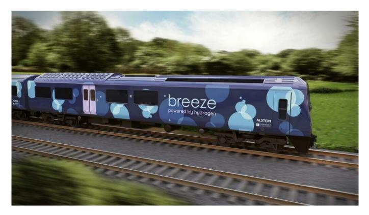
Alstom and Eversholt Rail have unveiled the design of a new hydrogen train for the UK market. The train, codenamed 'Breeze', will be a conversion of existing Class 321 trains, reengineering some of the UK's most reliable rolling stock, to create a clean train for the modern age. These trains could run across the UK as early as 2022, emitting only water and no harmful emissions at all.
