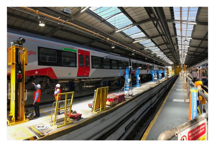
A new train lifting facility has been installed at Greater Anglia's Clacton rail depot to accommodate the operator's fleet of Stadler bi-mode trains – even though lockdown almost threw the project into jeopardy.
