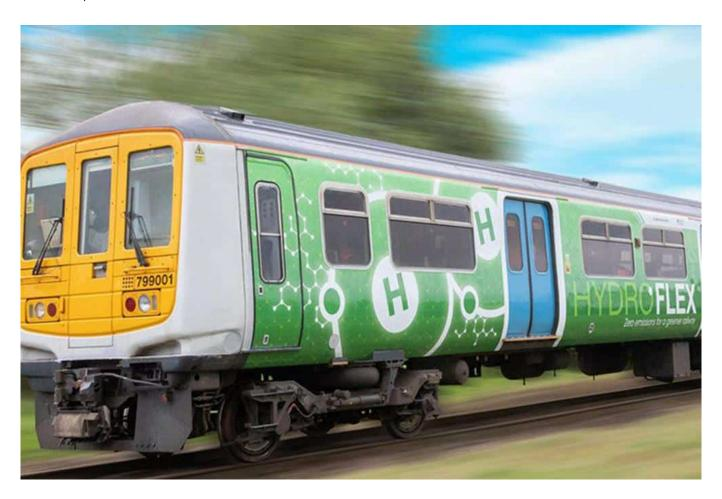
Mainline testing has begun for HydroFLEX, the first hydrogen-powered train to run on the UK's mainline. Danfoss Editron has supplied a converter, which is connected to the train's fuel cell provided by Ballard Power Systems.
