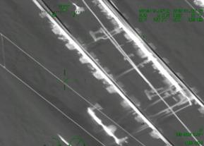
Thermal imaging cameras mounted to a Network Rail helicopter are keeping passengers and freight moving after heavy snowfall across the West Midlands.
