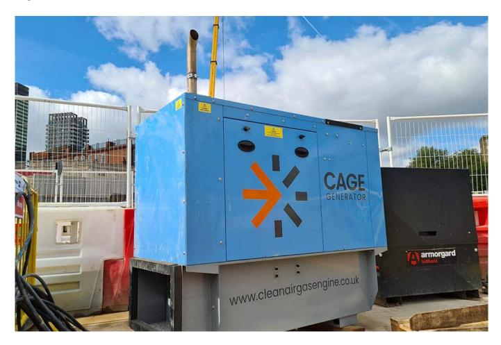
Following the successful trial of the new Clean Air Gas Engine (CAGE) integrated into a solar-battery hybrid power system in an Advante welfare unit on an HS2 construction site from December 2020, HS2 is trialling an OakTec standalone CAGE generator which has delivered massive reductions in emissions, resulting in improved air quality.
