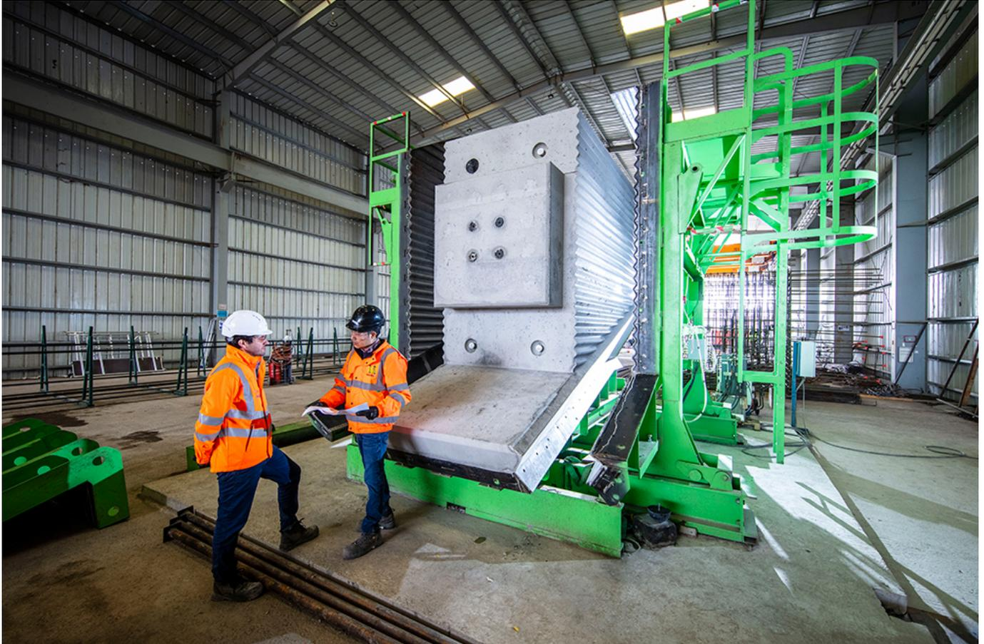
HS2 has revealed the first of 68 giant piers that will support the high speed rail project's first entirely off-site manufactured modular viaduct, in a move that represents a major step forward for viaduct design in the UK.
