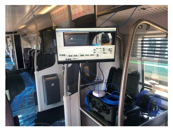
The first weekend in May saw a team drawn from Porterbrook, PCMS, Great Western Railway, Bombardier and DB Cargo (supported by ROG) successfully complete a further suite of European Train Control System (ETCS) tests on an eight car GWR Class 387 train operating on the main line between Reading and Heathrow.
