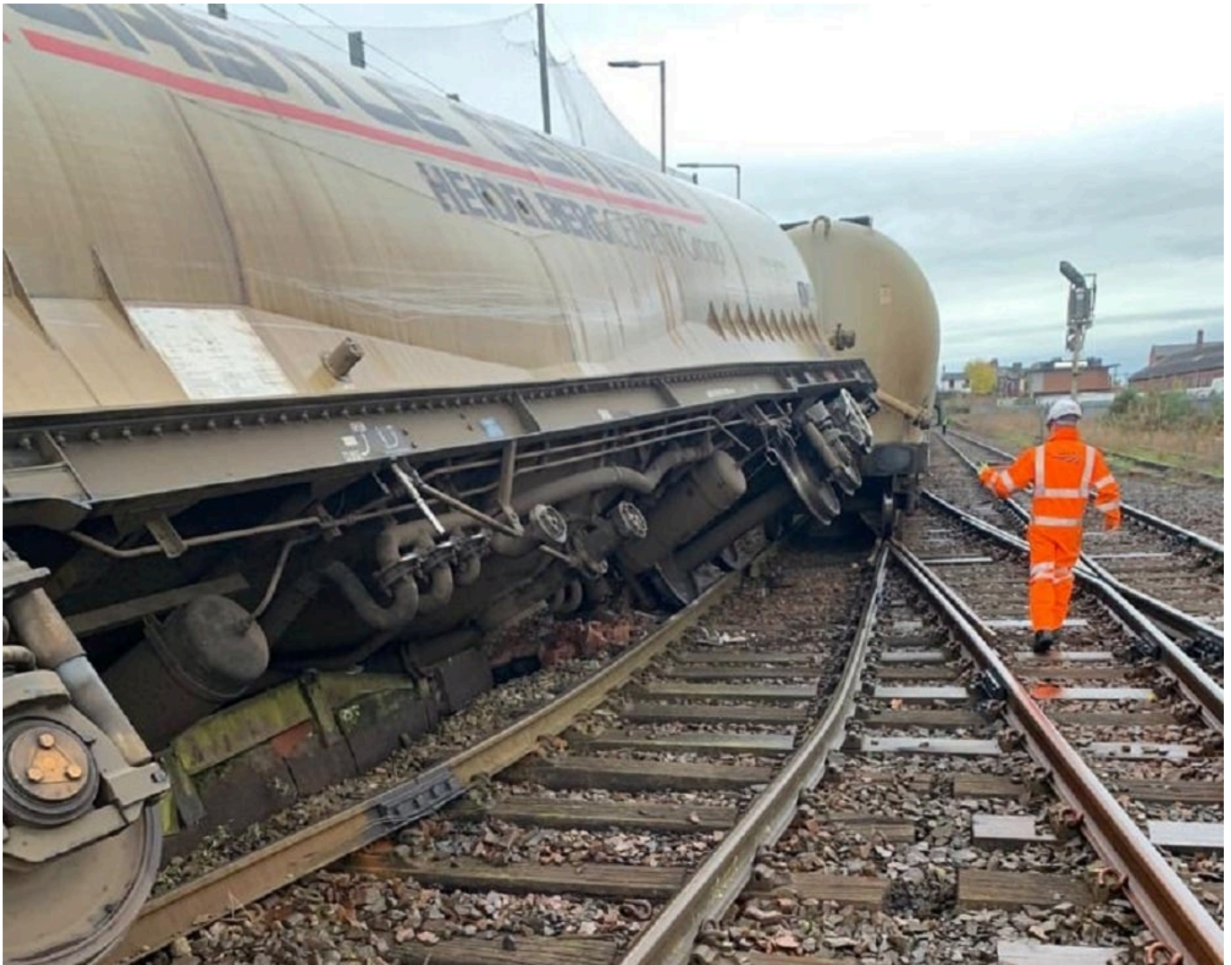
Track view of the derailed freight wagon
