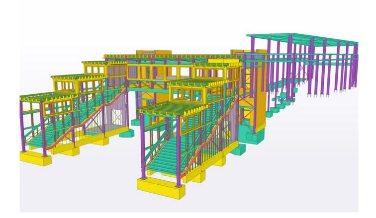
Discussing the refurbishment, Suj said: "This was a particularly challenging build at a busy operational London railway station. We developed a modular design strategy that would allow the structures to be installed over a series of single night line closures to minimise disruption at the station. Also allowing us to build majority of the concourse during days, so allowing the station to remain open to the public."
