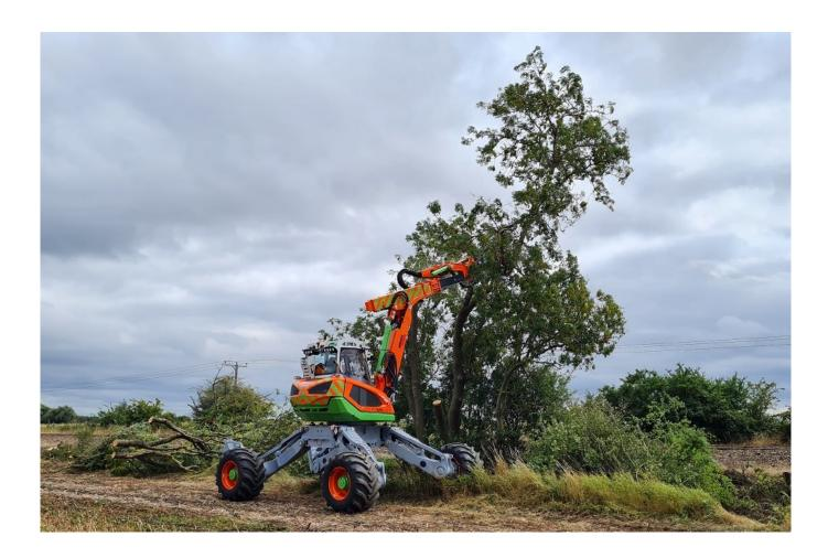
A great example of this was a recent river clearance for Severn Trent. To minimise disturbance to spawning trout and safely clear a build-up of debris around a sewer pipe, the Menzi Muck was deployed to travel through the stream, to clear the blockage. This was successfully achieved in just one day.
