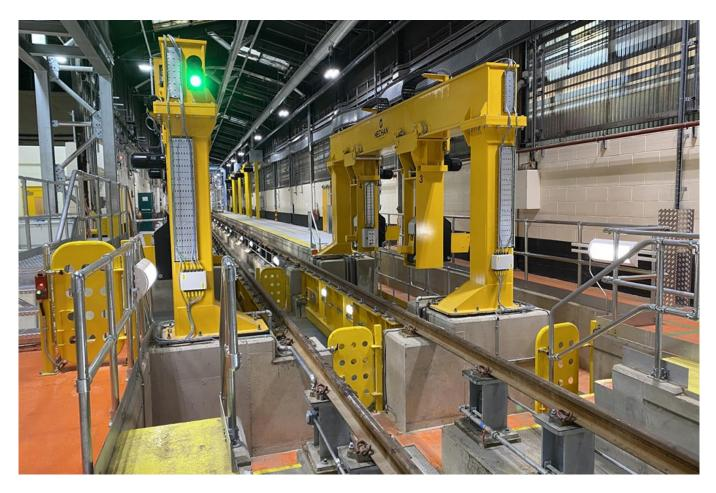
A new bogie drop facility has been installed at Greater Anglia's Crown Point rail depot to help maintain the operator's fleet of Stadler bi-mode trains.
