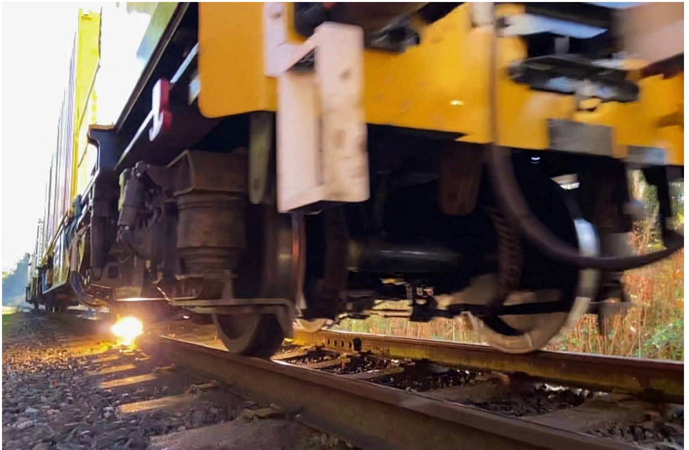
Side view of the plasma jet in action
