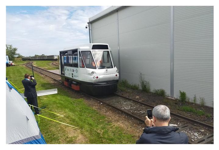
Pre Metro Operations has been playing its part in the development of a futuristic light rail vehicle that incorporates the use of Biomethane and kinetic energy storage.
