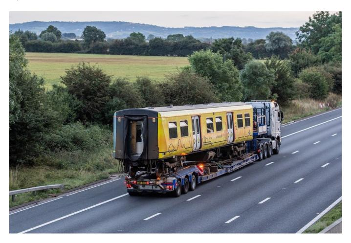
A three-car train heading down the M6 and M5 motorways perhaps raises questions in the minds of passing drivers: why are they on the motorway and where are they going? This was part of a complex move by Railway Support Services (RSS) of a class 507 EMU from Kirkdale depot to Newport Docks where the vehicles are to be dismantled.
