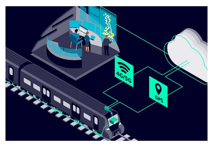
Siemens Mobility's train-borne conditioning monitoring (TBCM) system will play a part in Network Rail's Lot 1 Operational Trial, which has been established to assess means of predicting rough rides which are currently reported by drivers.
