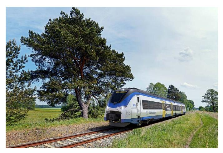
Siemens Mobility has been commissioned by Niederbarnimer Eisenbahn (NEB) to deliver seven two-car Mireo Plus H trains for the Heidekrautbahn network (RB27) in the Berlin-Brandenburg metropolitan region. Equipped with a fuel cell drive system and a lithium-ion battery, this second-generation hydrogen train provides completely CO<sub>2</sub> emission-free mobility.
