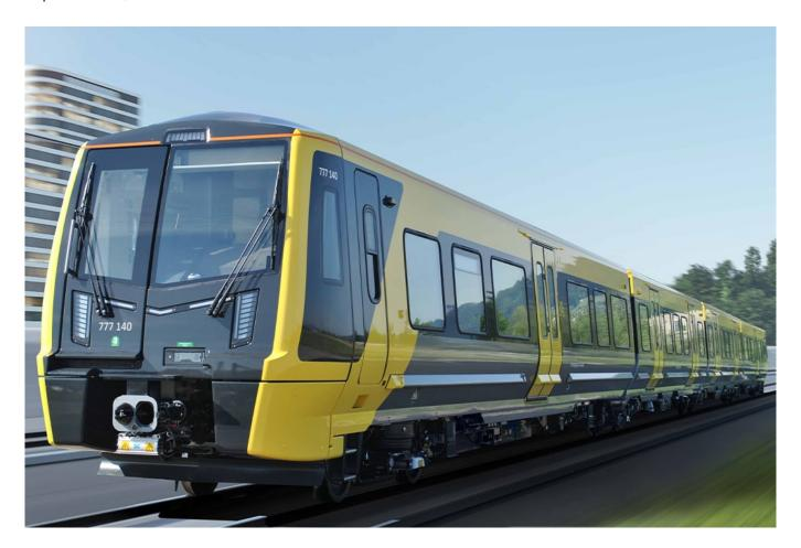
A Class 777/1 independently powered electric multiple unit (IPEMU), powered by battery, is one of seven vehicles that Stadler is displaying at InnoTrans this week in Berlin.
