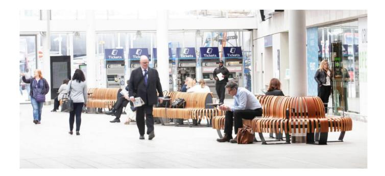
The station furniture comes with outstanding green credentials. At Liverpool Street the wooden seats themselves are oak and beech from 100 per cent FSC certified sources, the legs are 85 per cent recycled steel and the feet are made from recycled ocean plastic.
