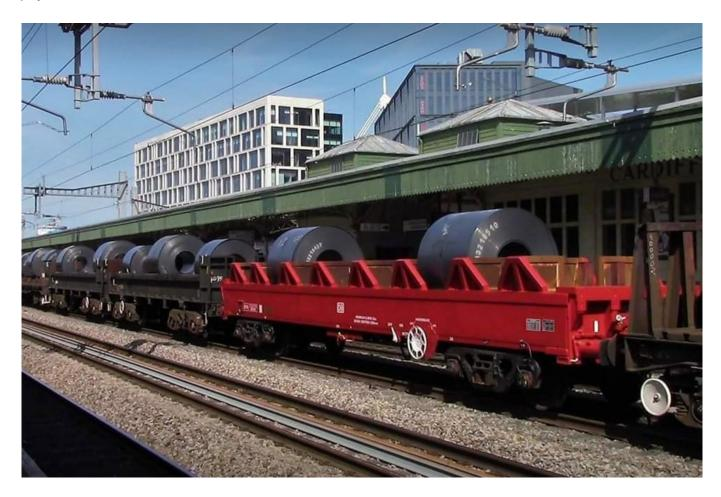
Innovative engineers at DB Cargo UK's maintenance depot in Stoke are busy converting a set of unused BYA wagons into open hot coil wagons-dubbed 'The Stegosaurus' due to its striking profile.
