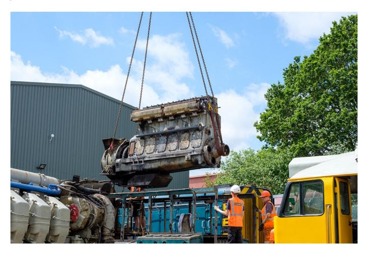
The Severn Valley Railway is celebrating the successful completion of the latest stage of its Harrier Hydroshunter project, with the removal of the original diesel engine from a Class 08 'donor' shunter.
