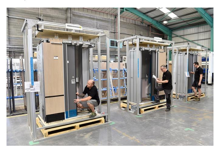
TRB Lightweight Structures is starting a new project as part of its long-term partnership with Hitachi, a global transport specialist at the forefront of innovation in the rail industry. The project involves the manufacture of toilet panels, partitions and doors, as well as modified bike and bulk units, for 23 new trains which are due to enter service by 2022.
