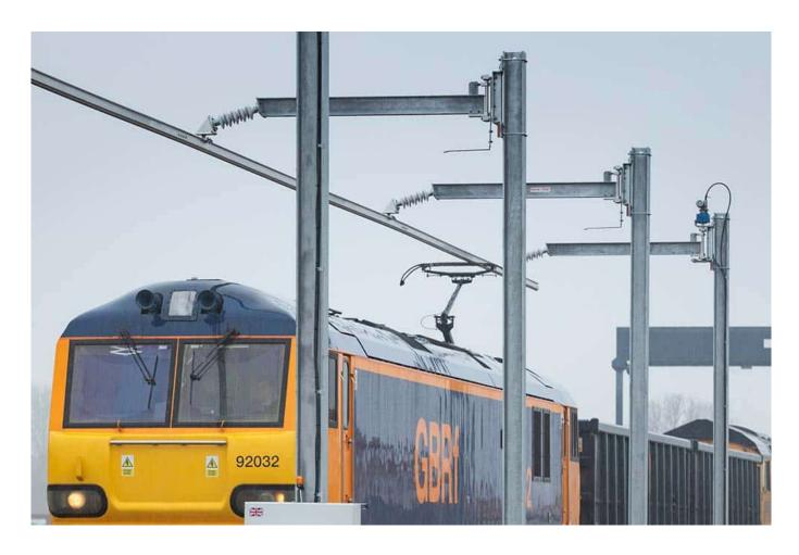
An innovative overhead electrification system could spell the end for diesel on electrified rail routes and boost the industry's net zero ambitions. Image Credit: Furrer+Frey
