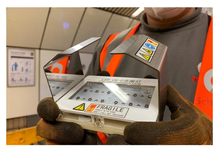
A new device that uses ultraviolet light to sanitise escalator handrails has been installed on the Tyne and Wear Metro as part of its range of COVID-secure measures.
