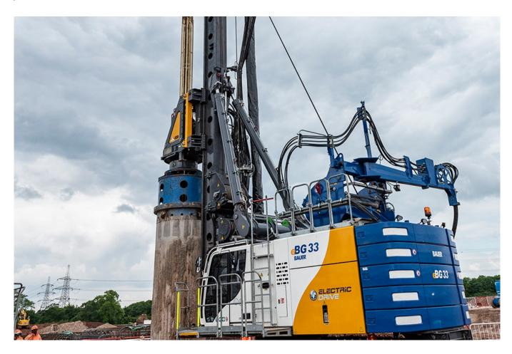
HS2 Ltd's construction partner Balfour Beatty VINCI Joint Venture (BBV), is trialling the world's first allelectric, high-capacity drilling rig on a construction site in Warwickshire, as the Joint Venture steps up its plans to meet HS2 Ltd's ambition for diesel-free construction sites.
